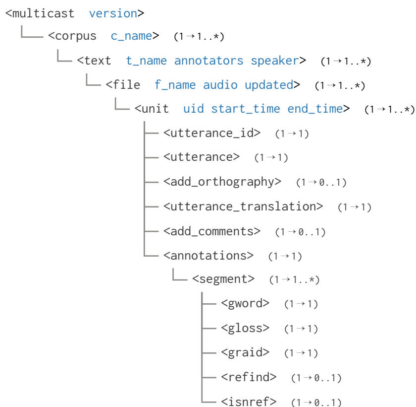
Figure 3 The structure of the Multi-CAST XML files. Attributes are given in blue. Cardinalities: (0..1) ‘zero or one’, (1) ‘exactly one’, (1..*) ‘one or more’.
